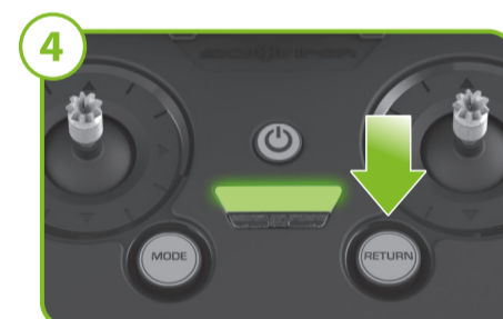
4 When flying in GPS mode, press the RETURN button to RETURN HOME. The frame will fly back to the home location and land. RETURN HOME will ONLY work if GPS LOCK is active.
