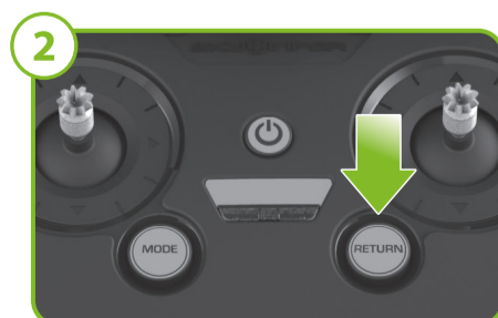
2 When flying in INDOOR mode, the RETURN button will cause the drone to LAND at its current location.
