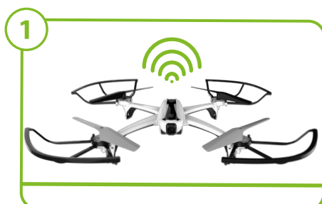
1 The frame will start to acquire GPS satellites. During this time, the GPS LOCK LED will blink.
