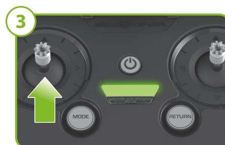
3 Raise the throttle stick to arm the frame. The motors will spin, indicating the frame is armed. Increase throttle to lift off of the ground.
