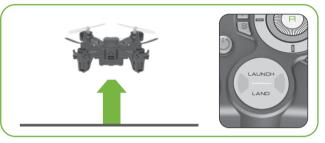
Press LAUNCH to automatically launch a few feet off the ground.
