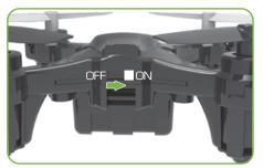
Turn the drone on. (Be sure that drone is completely charged. See reverse.)
