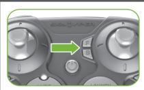
IF THE DRONE DRIFTS FORWARD: Press "B" button several times until the drone stops drifting forward
