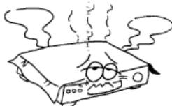
Do not block ventilation holes of the Receiver so that air can circulate freely.
