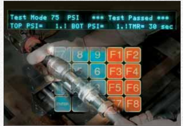
Repetitive testing ensures the leak-free integrity of every Galaxy boiler shipped.
