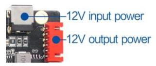
Power socket interfaces are defined as follows, can use power panel power supply, the socket specifications is 6 pin 2.54 mm spacing.
