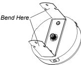
3. Connect the RG-59 cable to the F-type jack on the ceiling sensor.
