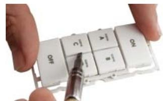
Please note that behind the buttons are clear plastic filler pieces; these diffuse the the buttons' LEDs' lights more elegantly. Use care to keep these filler pieces in the button frame as you reassemble the keypad.
