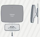
Slide the mount onto the back of the gateway. Tighten the screw located in the bottom of the mount.
