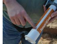
Figure 2: Showing the sensor snapped into the mounting bracket assembly with the white stripe facing up.
