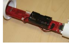
Figure 1: Inside panel of sensor showing where to install "AA" batteries.
