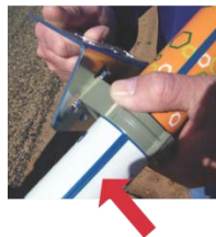
Figure 1: Showing the placement of clamp on bracket and the blue stripe on Field Sensor facing up.
