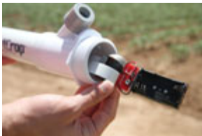
Figure 1: Inside battery clip of a Vertical Sensor showing where to install "AA" batteries.
