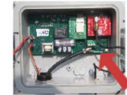
Figure 3: Showing the Battery & Solar Panel power cords plugged into the motherboard labeled “Battery” and “Solar Panel” pins.
