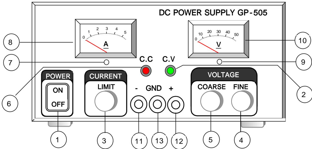
1. POWER SWITCH : This switch turns on and off the power.
