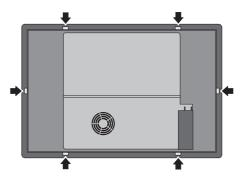
To install the clips into the hob, all you have to do is insert them horizontally into the appropriate space by applying light pressure.
