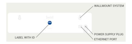
**Plug in** the Counter using the power cable and the adaptor provided.
