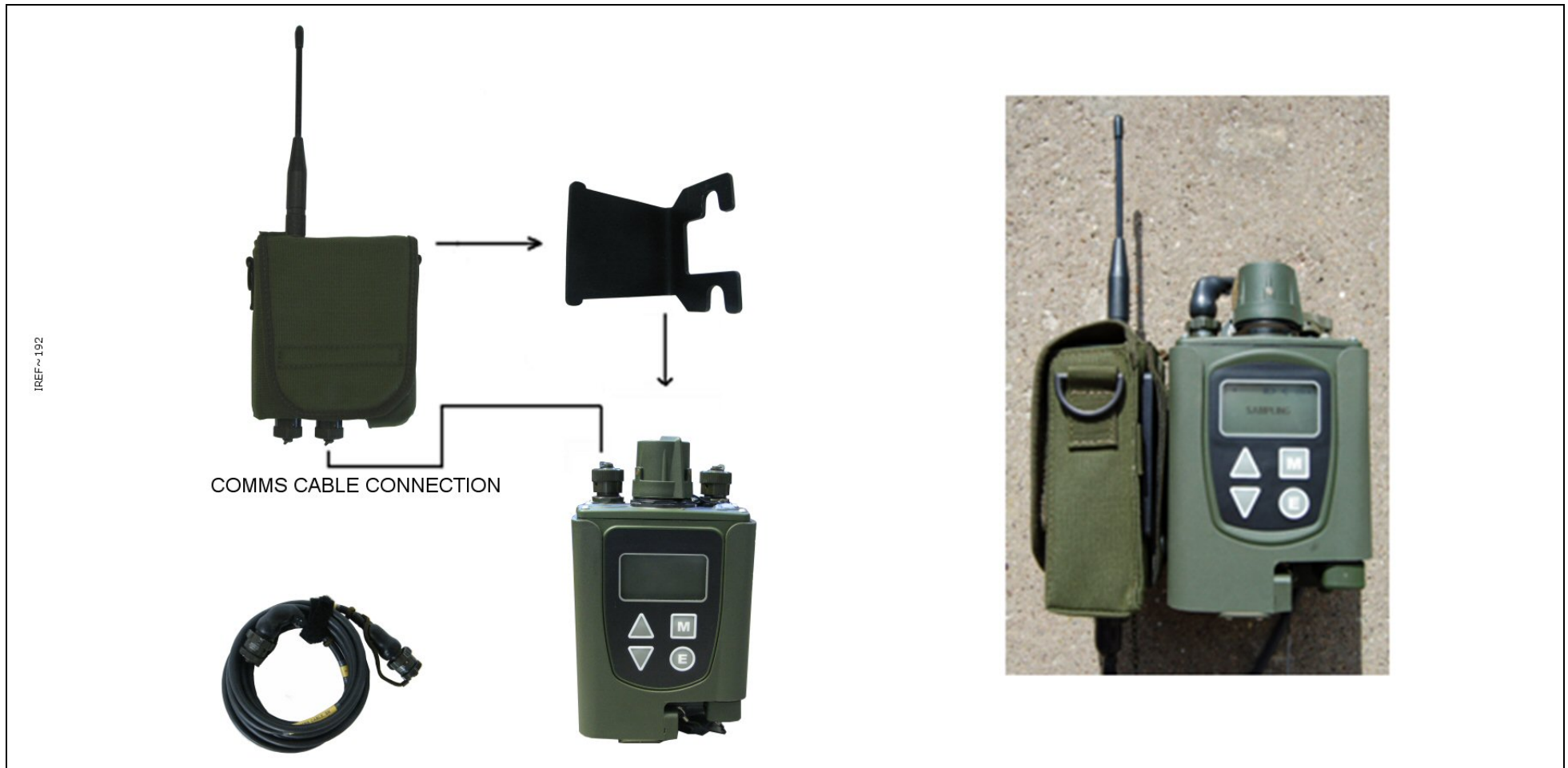
Figure 20 - Sensor Node with LCD3.3 and Power Comms Adaptor Set Up
