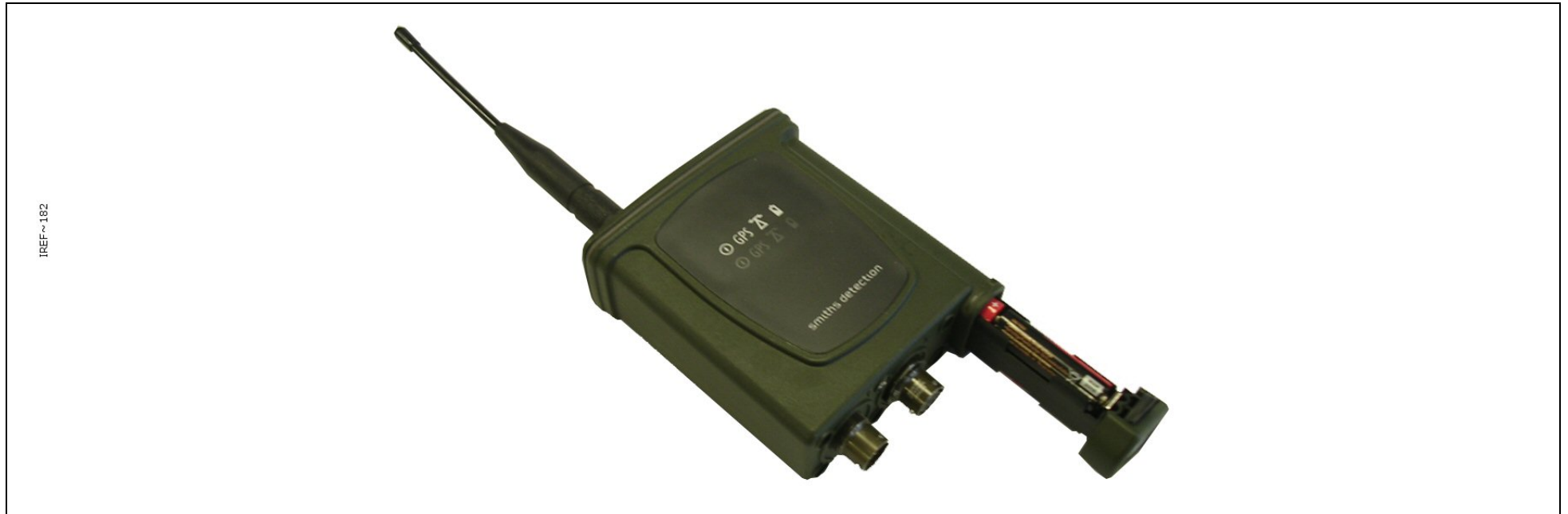
Figure 2 - Sensor Node (Battery Insertion)
