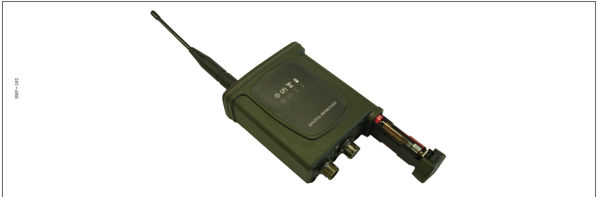
Figure 19 - Sensor Node (Battery Insertion)
