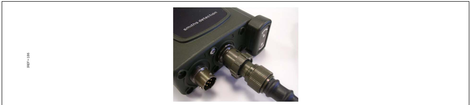
Figure 4 - Base Station Sensor Node Cable Connection
