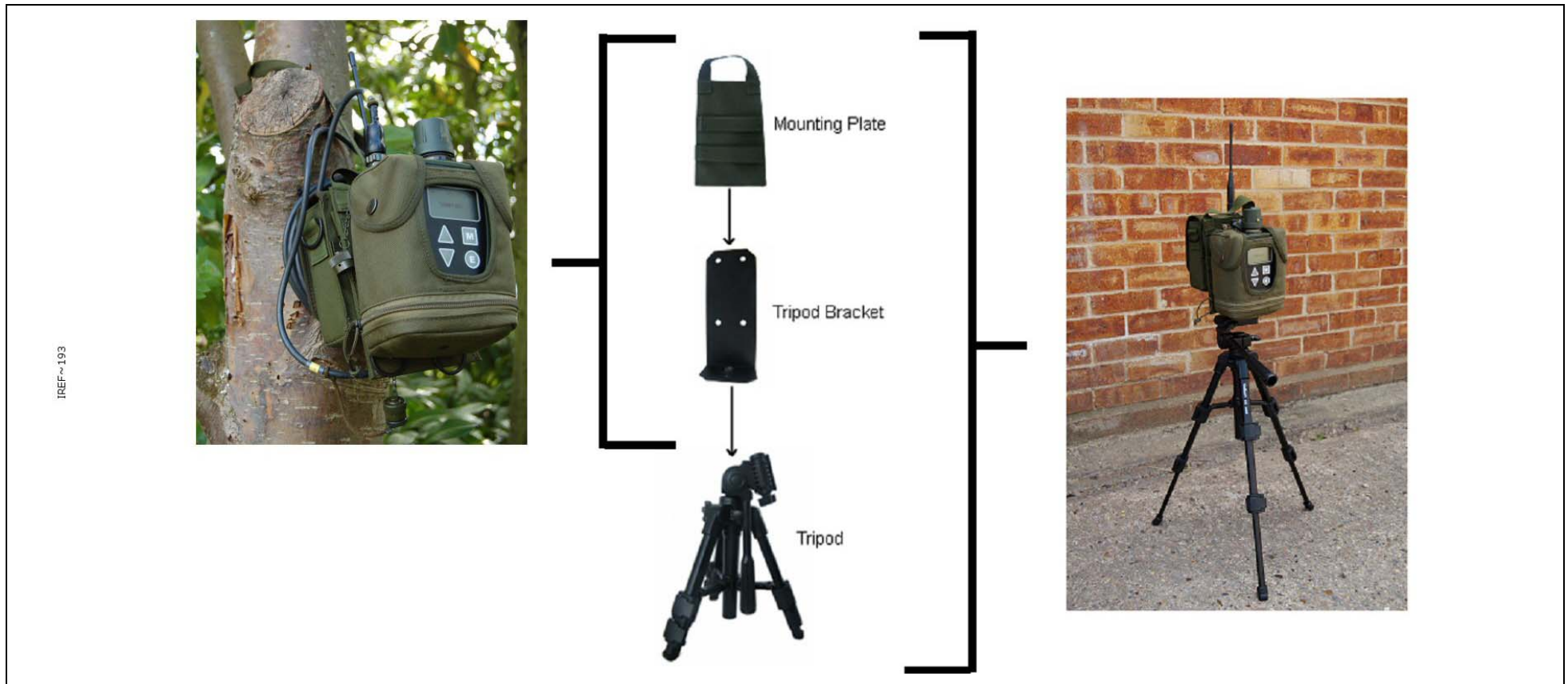
Figure 21 - Sensor Node with LCD3.3 and Power Comms Adaptor Set – in situ examples
