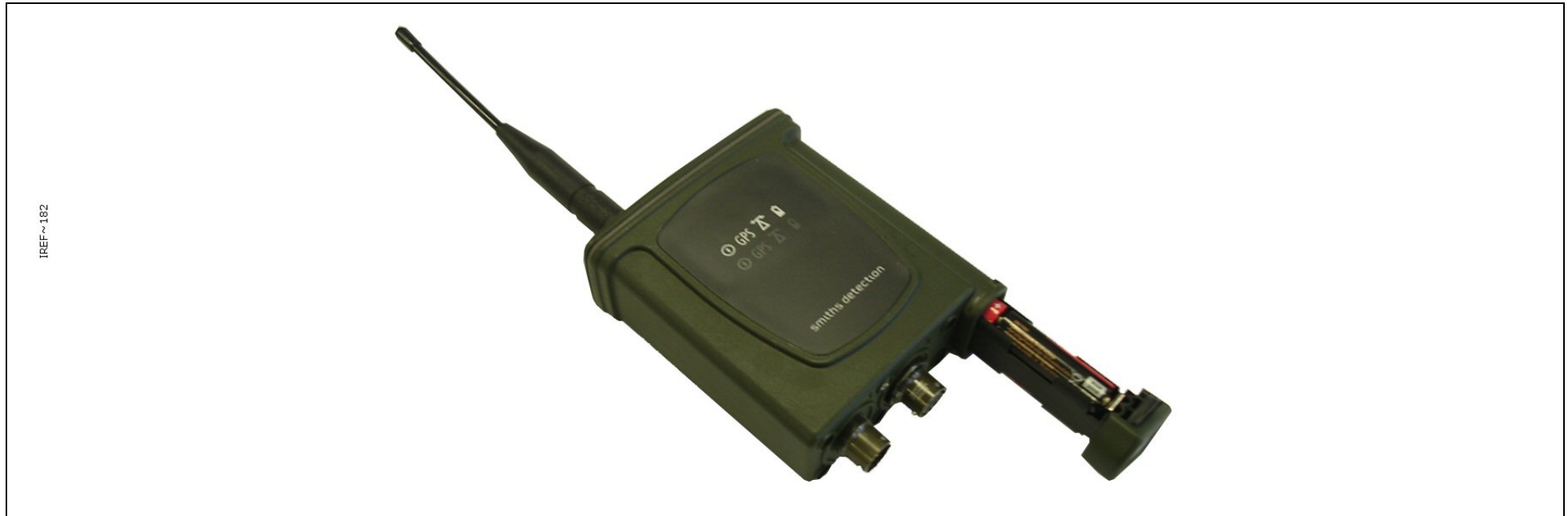
Figure 16 - Sensor Node (Battery Insertion)
