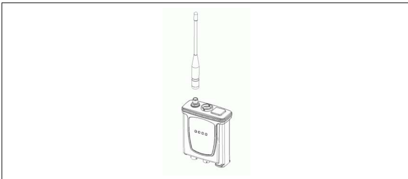
Figure 63 Radio Modem Antenna Replacement
