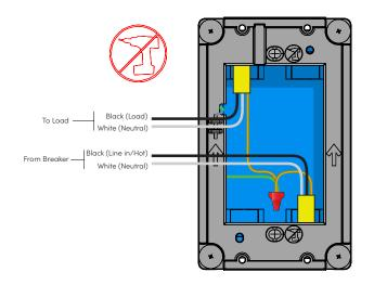
7 Identify and connect the wires to the back of the device. Insert the wire into the terminal and secure it by hand-tightening the set screw.
