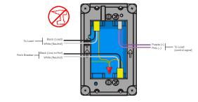
Identify and connect the wires to the back of the dimmer. Insert the wire into the terminal and secure it by hand-tightening the set screw.
