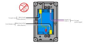
Identify and connect the wires to the back of the dimmer. Insert the wire into the terminal and secure it by hand-tightening the set screw...
