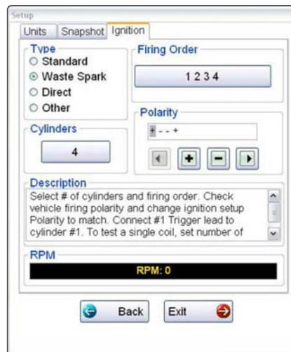
Figure 8-29 Sample Setup Ignition dialog box
