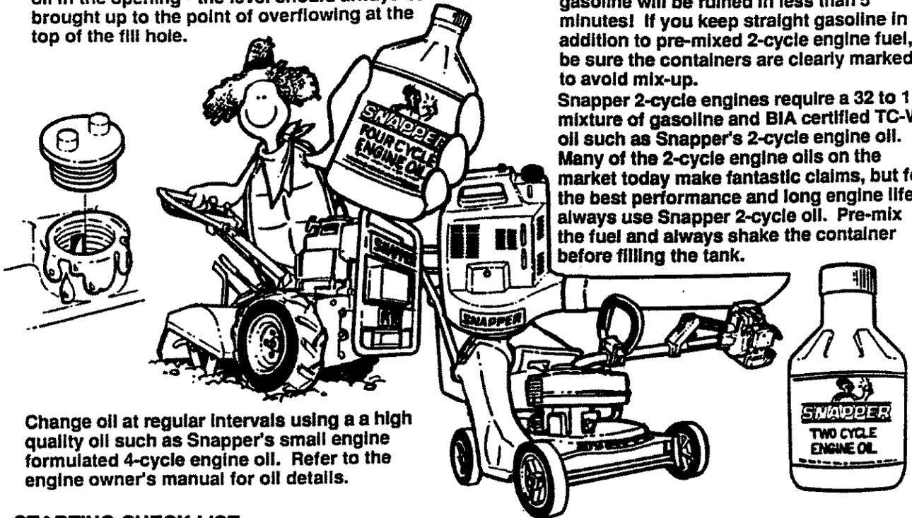
On 2-cycle engines, lubrication must be provided by an exact mixture of gasoline and 2-cycle air-cooled engine oil. A 2-cycle engine that is mistakenly run on straight gasoline will be ruined in less than 5 minutes! If you keep straight gasoline in addition to pre-mixed 2-cycle engine fuel, be sure the containers are clearly marked to avoid mix-up.
