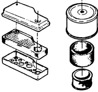
Generally, wash foam-type filters in a dishwashing detergent and water solution. Rinse and wring dry, then saturate with oil and squeeze out excess. *Failure to re-oil this type filter will ruin the engine.*
