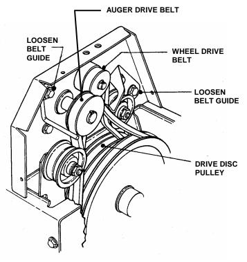
**5.** Tilt machine forward to gain access to drive system area. Secure machine in the tilted position to prevent tipping over. Remove drive system cover plate. See Figure 4.7.
