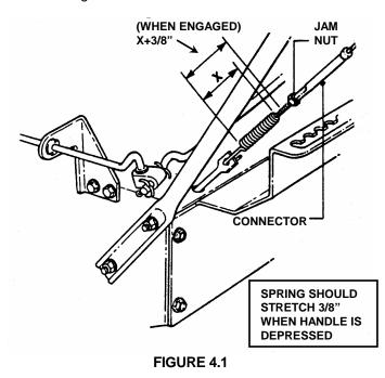
**2.** Adjust control cable by loosening jam nut at the upper end of cable. Hold threaded end of cable and then turn cable clockwise or counter clockwise until correct extension is achieved. Retighten jam nut.
