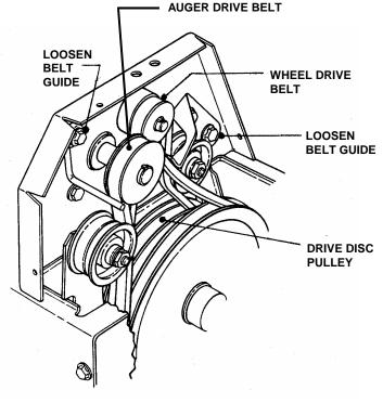
**5.** Tilt machine forward to gain access to drive system area. Secure machine in the tilted position to prevent tipping over. Remove drive system cover plate. See Figure 4.5.
