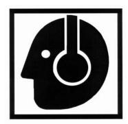
HEARING PROTECTION REQUIRED. Machine exceeds 100Lwa. MAXIMUM HANDLE VIBRATION 34 M/SEC<sup>2</sup>.
