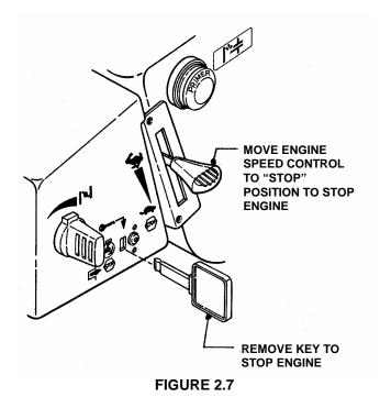
2.2 STARTING, OPERATION & STOPPING (ELECTRIC START MODELS) (Go to Page 8 for Recoil Start Models)
