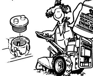
Change oil at regular intervals using a a high quality oil such as Snapper's small engine formulated 4-cycle engine oll. Refer to the engine owner's manual for oil details.
