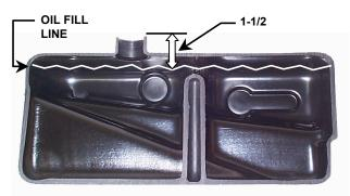
HYDRAULIC OIL RESERVOIR IMPORTANT: FLUID LEVEL MUST BE ABOVE TOP OF BAFFLE. RESERVOIR CAPACITY IS ONE (1) GALLON. <u>DO NOT OVERFILL</u>.
