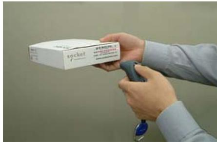
*When data is read and sent to the CK30, the scanner beam will turn off. Depending on your scanner settings, the scanner may beep and/or the CHS LED may flash green to indicate a good read.*
