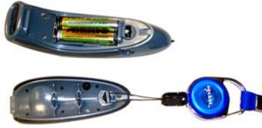
2. Install the batteries in opposite directions, as indicated by the positive symbols.
