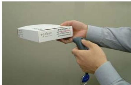
*When data is read and sent to the mobile computing device, the scanner beam will turn off. Depending on your scanner settings, the scanner may beep and/or the CHS LED may flash green to indicate a good read. If no data is read in a few seconds, the laser will turn off, and you must try again.*
