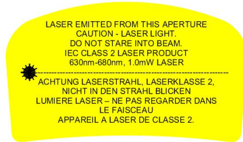
Example of Class 2 Laser Warning Label
