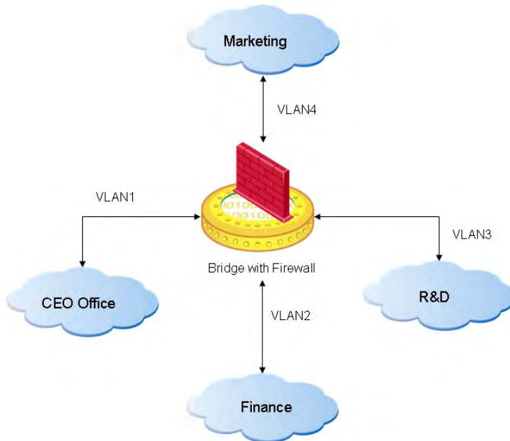
Figure 19: Bridge with Four VLANs
