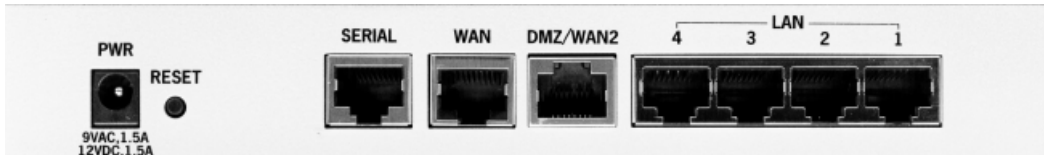
Figure 1: Safe@Office 500 SBX-166LHGE-5 Appliance Rear Panel
