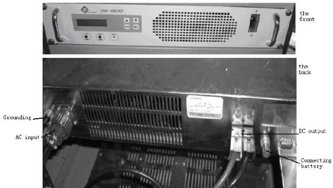
Fig 2-9: An example of a stand alone power supply to be installed in the cabinet
