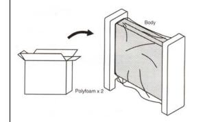
2. Remove the poly foam from both ends and remove the poly bag.
