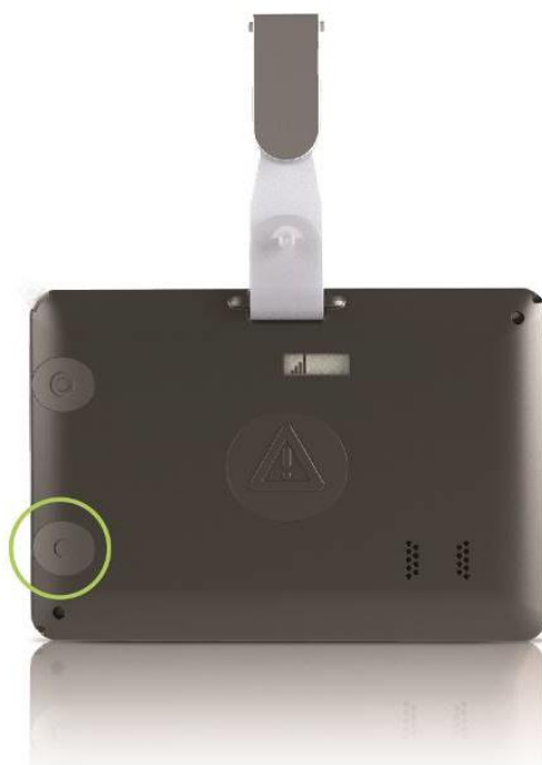
Figure 8: SoloProtect ID Amber Alert (Status Check in the USA and Canada)
