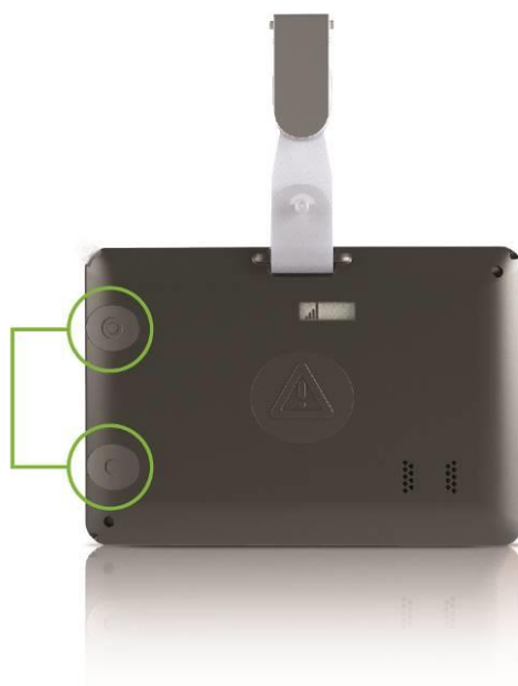
Figure 6: Turning your SoloProtect ID On and Off
