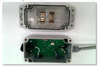
7. Place a battery between the two clips on the bottom portion. Make sure that the leads exiting the battery are in the 12 o'clock position.
