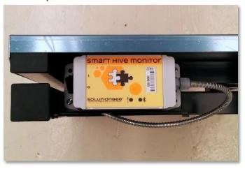
2. Remove the top plate. Identify the two screws (and washers and nuts) that attach the electronic module to the frame bracket.
