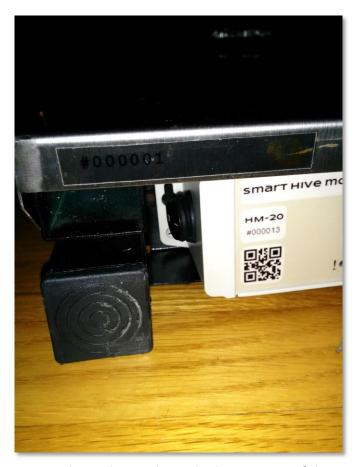
3. Zeroing the scale: Without the hive on top of the monitor, zero out the scale by pressing the orange button for between 5 and 20 seconds. The yellow warning light will blink for two seconds indicating that zeroing was successful.
