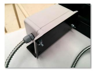
13. Reattach the top cover. You are done. Turn the power switch to the on - "I" position. Try to communicate with the module with an iPad as per the Installation Guide.
