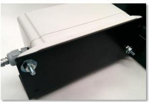
3. Remove the two bracket screws. The electronic module will now be free from the scale frame. Identify the four screws that hold the module together.
