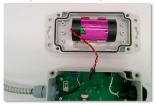
8. Insert the battery lead male connector into to mating female connector on the printed circuit board.
