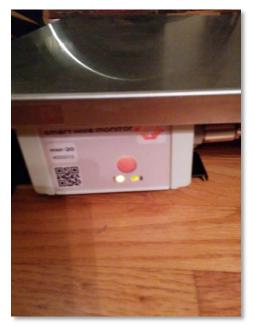
4. Place the beehive centered on top of the SHM. Make sure the ON/OFF switch remains in the ON position.
