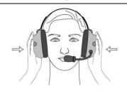
Test seal by pressing against your head and listening for a change in sound level
