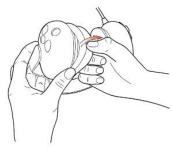
2. Starting at the bottom, place the new ear seal on the dome. Pull over the lip of the ear dome using your finger. Do not use any sharp tool as it may damage the ear seal and reduce hearing protection.
