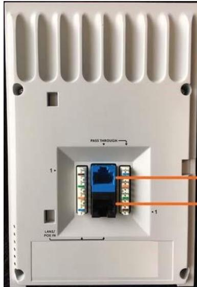
The bottom edge provides more ports. The blue Pass Through port is directly connected to the blue Pass Through port on the back panel of the unit, allowing you to connect to a second network available in the same wall jack that provides your PoE-enabled network connection.
