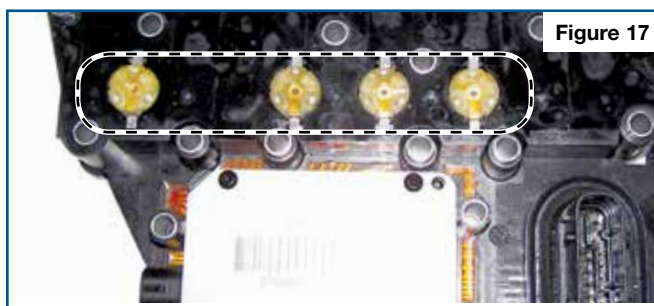
Generation 1, Control Solenoid (w/body and TCM) Valve Assembly: 4 Pressure Switches
