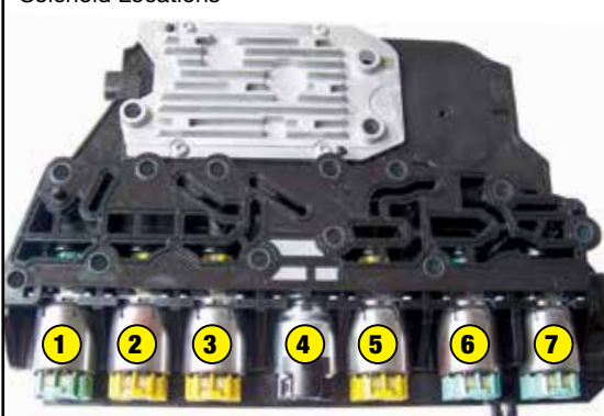
6T40 Generation 2 Solenoid Locations
