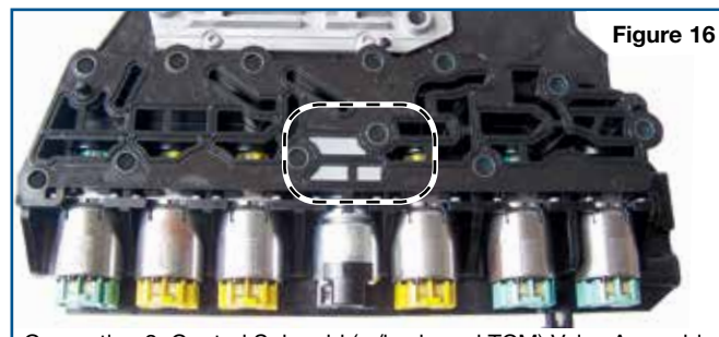
Generation 2, Control Solenoid (w/body and TCM) Valve Assembly, Beaded gasket and screen changed. Solenoid caps changed color.
