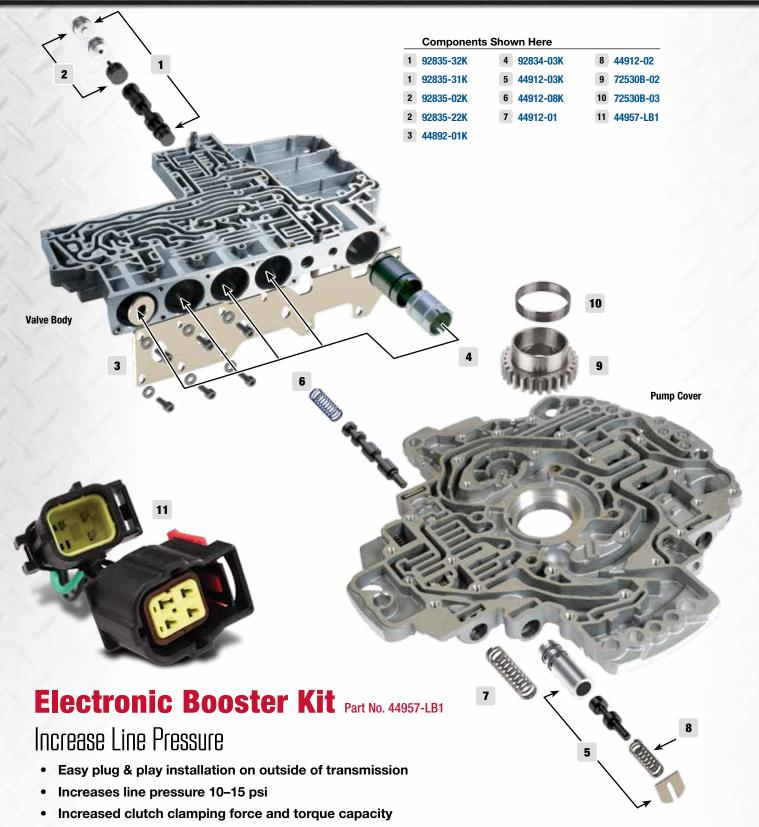
Sonnax electronic booster kits modify the line pressure sensor signal that causes the computer to increase pressure. This is an ideal upgrade for a little extra pressure in aggressive driving or loaded conditions.
