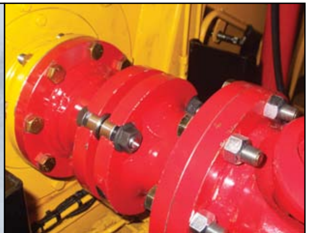
Shown above is a Power Train Saver industrial unit installed in the Snow Wolf SB-1050, a high-speed, high-capacity airport snow blower by Airport Technologies in Manitoba, Canada.
