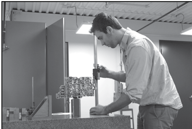
The facility features several testing rooms where our engineers can test and retest every necessary measurement on a new product. Here, Neal gets precision measurements on a valve body casting.
