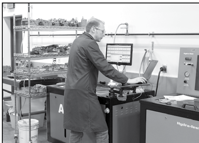
Above, two Sonnax engineers test a couple of valve bodies. On the left, Zach is utilizing one of the valve body testing machines. On the right, John is prepping a valve body for test.
