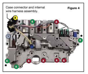
e. When reinstalling valve body, first temporarily tighten the two bolts marked (★) in **Figure 4** as they are positioning bolts.
