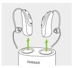
(i) Do not hold the tubes for removing the hearing aids from the charger as this can damage the xReceiver.
