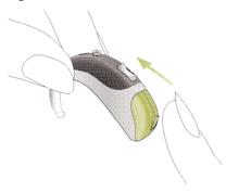
Close the battery compartment. Your Naída hearing systems are always working in the initial hearing program, and at the preset volume when turned ON.
