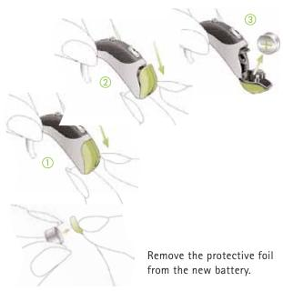
Insert the new battery with the "+" sign (flat side of the battery) in line with the "+" marked on the battery cover ④, ⑤. Push the battery door upwards to close it
