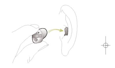
Grasp the hearing system between the thumb and index finger, using the hand on the same side you wear your hearing system. Insert the canal end into the ear canal. Tug gently on your ear lobe and push the hearing system into the correct position.
