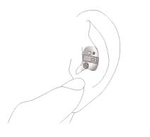
• Exélia or Exélia Petite without a removal handle Put your thumb behind your lobe (just below the hard cartilage) and gently press your ear upward to push the hearing system out of the canal. In order to help it along, make chewing movements with your jaw.
