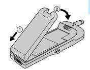
2 Attach the battery pack by pressing down firmly on the thumb indent.
