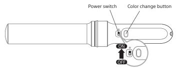
② Except while wireless signals are being received, the color of the light changes to a preset light color each time the color change button is pressed.
