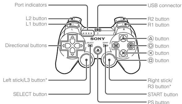
\* The L3 and R3 buttons function when the sticks are pressed.
