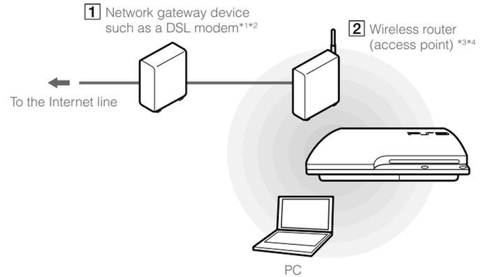
\*1 The connection method may vary depending on the environment in use. For example, you may be able to connect Ethernet cables directly into the wall outlet in housing complex units that have preinstalled LAN ports. If you are using such a network environment, you do not need a network gateway device.
