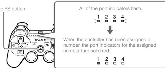
You can connect up to 7 controllers at one time. The controller number is shown by the number above the port indicators. For numbers 5-7, add the numbers of the lit indicators.
