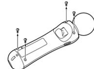
**3 Carefully remove the casing. 4 Unplug the connector, and then remove the battery.**
