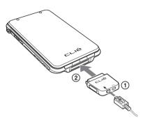
**2** Connect the "A" plug of the USB cable to the USB port of your computer.
