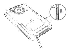
**3** Wait for more than three seconds after the **palm** POWERED screen is displayed, and release the POWER/ HOLD switch.
