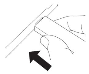
4. While pressing and holding the SHARE button on the controller, press and hold the @ (PS) button for at least 3 seconds.
