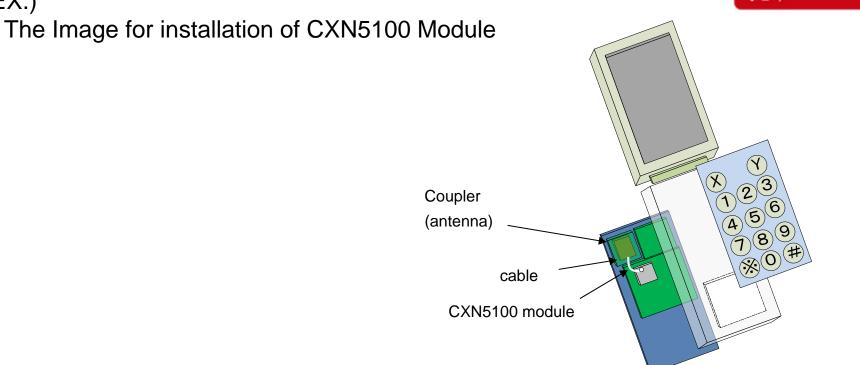
Only the coupler (LDA5M4G4815L-301 or LDA5M4G4820L-302) which received approval with CXN5100 can be used.
