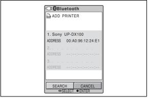
If one or two printers are still connectable, add printer(s) as shown in the following steps. If three printers are already connected, an unnecessary printer must be deleted beforehand.
