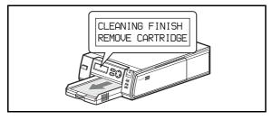
**7** Remove the cleaning cassette from the printer, and reinsert the print cartridge and paper tray.
